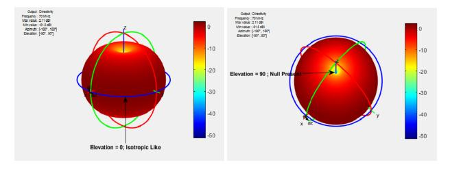
The dipole is omnidirectional around the E-plane, or elevation angle. The null is present in the H-plane, or azimuth angle.
